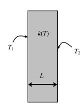
Then the rate of heat conduction through the plate becomes
