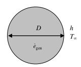
**2-152** A spherical reactor of 5-cm diameter operating at steady condition has its heat generation suddenly set to 9 MW/m<sup>3</sup>. The time rate of temperature change in the reactor is to be determined.
