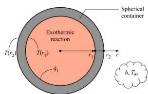
**2-76** A spherical container is subjected to uniform heat flux on the outer surface and specified temperature on the inner surface. The mathematical formulation, the variation of temperature in the pipe, and the outer surface temperature, and the maximum rate of hot water supply are to be determined for steady one-dimensional heat transfer.
