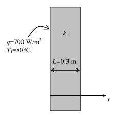
**2-58** The base plate of a household iron is subjected to specified heat flux on the left surface and to specified temperature on the right surface. The mathematical formulation, the variation of temperature in the plate, and the inner surface temperature are to be determined for steady one-dimensional heat transfer.
