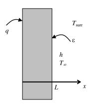
**2-144** A large plane wall is subjected to convection on the inner and outer surfaces. The mathematical formulation, the variation of temperature, and the temperatures at the inner and outer surfaces to be determined for steady one-dimensional heat transfer.
