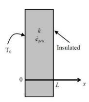
**2-88** Heat is generated in a large plane wall whose one side is insulated while the other side is maintained at a specified temperature. The mathematical formulation, the variation of temperature in the wall, and the temperature of the insulated surface are to be determined for steady one-dimensional heat transfer.
