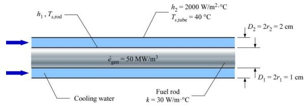
Analysis The rate of heat transfer by convection at the fuel rod surface is equal to that of the concentric tube surface:
