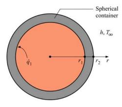
**2-74** A spherical container is subjected to specified temperature on the inner surface and convection on the outer surface. The mathematical formulation, the variation of temperature, and the rate of heat transfer are to be determined for steady one-dimensional heat transfer.
