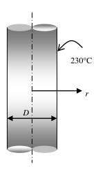
**2-93** Heat is generated in a long solid cylinder with a specified surface temperature. The variation of temperature in the cylinder is given by
