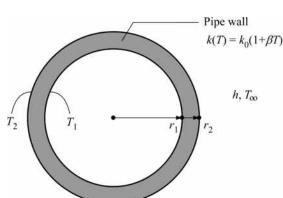
2-155 A metal spherical tank, filled with chemicals undergoing an exothermic reaction, has a known inner surface temperature. The tank wall has a variable thermal conductivity. Convection heat transfer occurs on the outer tank surface. The heat flux on the inner surface of the tank is to be determined.
