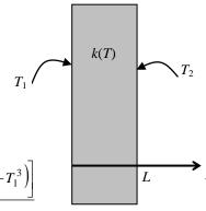
$$k_{\text{avg}} = \frac{\int_{T_1}^{T_2} k(T) dT}{T_2 - T_1} = \frac{\int_{T_1}^{T_2} k_0 (1 + \beta T^2) dT}{T_2 - T_1} = \frac{k_0 \left( T + \frac{\beta}{3} T^3 \right)_{T_1}^{T_2}}{T_2 - T_1} = \frac{k_0 \left[ \left( T_2 - T_1 \right) + \frac{\beta}{3} \left( T_2^3 - T_1^3 \right) \right]}{T_2 - T_1}$$
