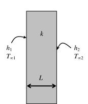
**2-145** A steam pipe is subjected to convection on both the inner and outer surfaces. The mathematical formulation of the problem and expressions for the variation of temperature in the pipe and on the outer surface temperature are to be obtained for steady one-dimensional heat transfer.
