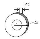
**2-34** Consider a thin disk element of thickness  $\Delta z$  and diameter D in a long cylinder. The density of the cylinder is  $\rho$ , the specific heat is c, and the area of the cylinder normal to the direction of heat transfer is  $A = \pi D^2 / 4$ , which is constant. An *energy balance* on this thin element of thickness  $\Delta z$  during a small time interval  $\Delta t$  can be expressed as
