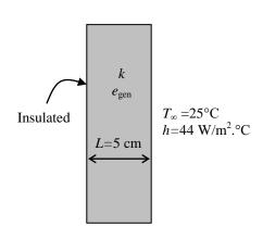
**2-84** Prob. 2-83 is reconsidered. The effect of the heat transfer coefficient on the highest and lowest temperatures in the plate is to be investigated.
