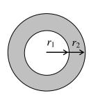
**2-49** A spherical shell of inner radius  $r_1$ , outer radius  $r_2$ , and thermal conductivity k is considered. The outer surface of the shell is subjected to radiation to surrounding surfaces at  $T_{\rm surr}$ . Assuming no convection and steady one-dimensional conduction in the radial direction, the radiation boundary condition on the outer surface of the shell can be expressed as
