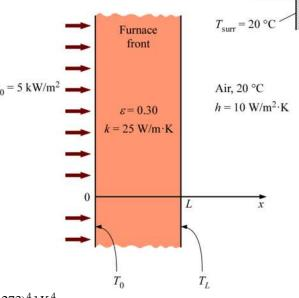
**2-65E** A large plate is subjected to convection, radiation, and specified temperature on the top surface and no conditions on the bottom surface. The mathematical formulation, the variation of temperature in the plate, and the bottom surface temperature are to be determined for steady one-dimensional heat transfer.
