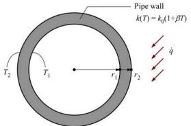
A pipe is used for transporting boiling water with a known inner surface temperature in surroundings of cooler ambient temperature and known convection heat transfer coefficient. The pipe wall has a variable thermal conductivity. The outer surface temperature of the pipe is to be determined to ensure that it is below 50°C.
