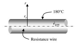
**2-100** A cylindrical fuel rod is cooled by water flowing through its encased concentric tube while generating a uniform heat. The variation of temperature in the fuel rod and the center and surface temperatures are to be determined for steady one-dimensional heat transfer.
