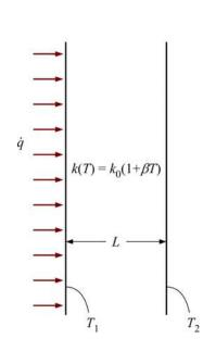
**2-112** A plate with variable conductivity is subjected to specified temperatures on both sides. The rate of heat transfer through the plate is to be determined.
