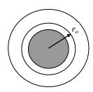
**2-51** A spherical metal ball that is heated in an oven to a temperature of  $T_i$  throughout is dropped into a large body of water at  $T_{\infty}$  where it is cooled by convection. Assuming constant thermal conductivity and transient one-dimensional heat transfer, the mathematical formulation (the differential equation and the boundary and initial conditions) of this heat conduction problem is to be obtained.
