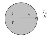
**2-52** A spherical metal ball that is heated in an oven to a temperature of  $T_i$  throughout is allowed to cool in ambient air at  $T_{\infty}$  by convection and radiation. Assuming constant thermal conductivity and transient one-dimensional heat transfer, the mathematical formulation (the differential equation and the boundary and initial conditions) of this heat conduction problem is to be obtained.
