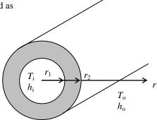
**2-146** A 10-m tall exhaust stack discharging exhaust gases at a rate of 1.2 kg/s is subjected to solar radiation and convection at the outer surface. The variation of temperature in the exhaust stack and the inner surface temperature of the exhaust stack are to be determined.
