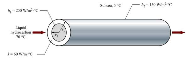
Analysis The inner and outer radii of the pipeline are
