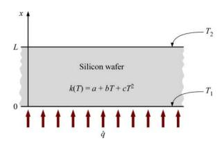
The maximum allowable heat flux such that the temperature difference across the wafer thickness does not exceeding 2 °C is
