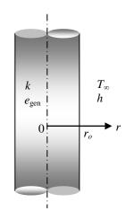
**2-99** A long homogeneous resistance heater wire with specified surface temperature is used to heat the air. The temperature of the wire 3.5 mm from the center is to be determined in steady operation.
