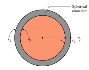
**2-73** A spherical shell is subjected to uniform heat flux on the inner surface, while the outer surface is subjected to convection heat transfer. The variation of temperature in the shell wall and the outer surface temperature are to be determined for steady one-dimensional heat transfer.
