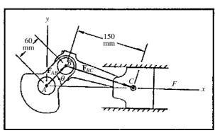
**Problem 2.33** In Example 2.4, the coordinates of the fixed point A are (17, 1) ft. The driver lowers the bed of the truck into a new position in which the coordinates of point B are (9, 3) ft. The magnitude of the force F exerted on the bed by the hydraulic cylinder when the bed is in the new position is 4800 lb. Draw a sketch of the new situation. Express F in terms of components.
