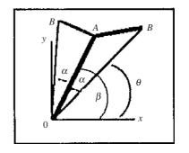
**Problem 2.35** The magnitude of the position vector  $\mathbf{r}_{BA}$  from point B to point A is 6 m and the magnitude of the position vector  $\mathbf{r}_{CA}$  from point C to point A is 4 m. What are the components of  $\mathbf{r}_{BA}$ ?
