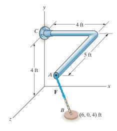
**Problem 2.127** The two segments of the L-shaped bar are parallel to the x and z axes. The rope AB exerts a force of magnitude  $|\mathbf{F}| = 500$  lb on the bar at A. Determine the cross product  $\mathbf{r}_{CB} \times \mathbf{F}$ , where  $\mathbf{r}_{CB}$  is the position vector form point C to point B. Compare your answers to the answer to Problem 2.126.
