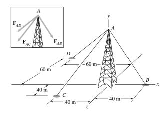
**Problem 2.94** Consider the tower described in Problem 2.93. The magnitude of the force  $\mathbf{F}_{AB}$  is 2 kN. The x and z components of the vector sum of the forces exerted on the tower by the three cables are zero. What are the magnitudes of  $\mathbf{F}_{AC}$  and  $\mathbf{F}_{AD}$ ?
