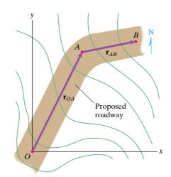
**Solution:** Two possibilities are: The point *B* lies west of point *A*, or point *B* lies east of point *A*, as shown. The strategy is to determine the unknown angles  $\alpha$ ,  $\beta$ , and  $\theta$ . The magnitude of *OA* is
