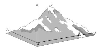
**Problem 2.83** The distance from point O to point A is 20 ft. The straight line AB is parallel to the y axis, and point B is in the x-z plane. Express the vector  $\mathbf{r}_{OA}$  in terms of scalar components.
