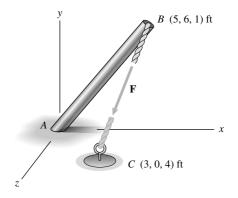
**Problem 2.159** The pole supporting the sign is parallel to the x axis and is 6 ft long. Point A is contained in the y-z plane. (a) Express the vector  $\mathbf{r}$  in terms of components. (b) What are the direction cosines of  $\mathbf{r}$ ?
