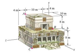
**Problem 2.80** Observers at A and B use theodolites to measure the direction from their positions to a rocket in flight. If the coordinates of the rocket's position at a given instant are (4, 4, 2) km, determine the direction cosines of the vectors  $\mathbf{r}_{AR}$  and  $\mathbf{r}_{BR}$  that the observers would measure at that instant.
