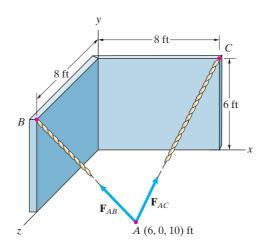
**Problem 2.92** Consider the cables and wall described in Problem 2.91. Cable AB exerts a 200-lb force  $\mathbf{F}_{AB}$  at point A that is directed along the line from A to B. The cable AC exerts a 100-lb force  $\mathbf{F}_{AC}$  at point A that is directed along the line from A to C. Determine the magnitude of the total force exerted at point A by the two cables.
