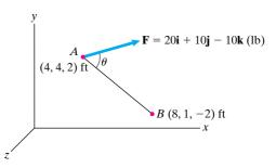
**Problem 2.152** Determine the scalar components of a unit vector parallel to line AB that points from A toward B.
