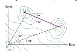
**Solution:** Draw the vectors accurately and then measure the unknown magnitude and angle.
