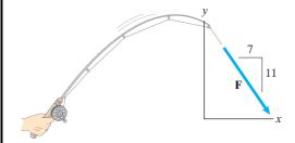
**Solution:** We can use similar triangles to determine the components of  ${\bf F}$ .
