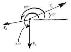
**Problem 2.50** Four forces act on a beam. The vector sum of the forces is zero. The magnitudes  $|\mathbf{F}_B| = 10 \text{ kN}$  and  $|\mathbf{F}_C| = 5 \text{ kN}$ . Determine the magnitudes of  $\mathbf{F}_A$  and  $\mathbf{F}_D$ .
