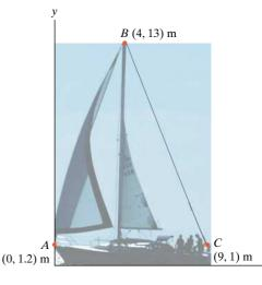
**Problem 2.108** Determine the angle  $\theta$  between the lines AB and AC (a) by using the law of cosines (see Appendix A); (b) by using the dot product.
