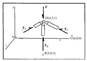
**Problem 2.162** The magnitude of the vertical force vector  $\mathbf{F}$  in Problem 2.161 is 6 kN. Determine the vector components of  $\mathbf{F}$  parallel and normal to the line from B to D.
