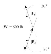
**Problem 2.12** The rope ABC exerts forces  $\mathbf{F}_{BA}$  and  $\mathbf{F}_{BC}$  of equal magnitude on the block at B. The magnitude of the total force exerted on the block by the two forces is 200 lb. Graphically determine  $|\mathbf{F}_{BA}|$ .
