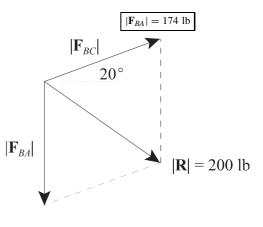
**Problem 2.13** Two snowcats tow an emergency shelter to a new location near McMurdo Station, Antarctica. (The top view is shown. The cables are horizontal.) The total force  $\mathbf{F}_A + \mathbf{F}_B$  exerted on the shelter is in the direction parallel to the line L and its magnitude is 400 lb. Graphically determine the magnitudes of  $F_A$  and  $\mathbf{F}_B$ .
