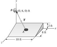
**Solution:** Consider a line on the sloped surface from *A* perpendicular to the surface. (see the diagram above) By SIMILAR triangles we see that one such vector is  $\mathbf{r}_N = 8\mathbf{j} + 2\mathbf{k}$ . Let us find the component of **F** parallel to this line.
