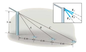
**Solution:** Use the angles and magnitudes to determine the vector components, take the sum, and solve for the unknown. The angles between each cable and the pillar are:
