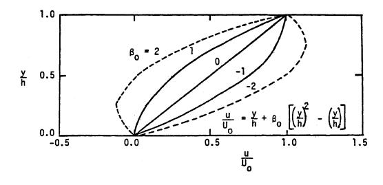
2.24 Contd.) The factor  $\frac{h^2}{2\mu U_0} \frac{dp}{dx}$  is a constant for a given problem, which we shall call  $\beta_0$ . The velocity profiles ( $u/U_0$ ) are presented in the sketch as a function of (y/h) for various values of  $\beta_0$ . Note that the profile is "fuller" when the pressure decreases in the x-direction, i.e.,  $\beta_0$  is negative, which is known as a favorable pressure gradient. If u=0, when  $y=\frac{h}{2}$
