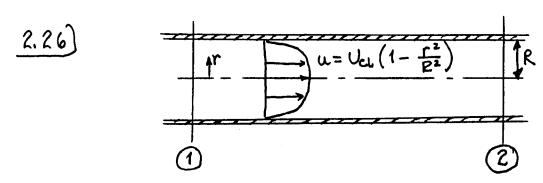
The first term on the right-hand side is zero for steady flow. The second term on the right-hand side is zero for fully-developed flow, since the efflux of momentum through the surface of the control volume (i.e., crossing station(2)) is of equal magnitude but opposite sign to the influx of momentum through the surface of the control volume (i.e., crossing station 1). To see that this is true, let us evaluate the second term on the right-hand side:
