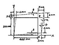
**Ans:**  $(\gamma_B)_{xy} = 11.6(10^{-3}) \text{ rad,}$   $(\gamma_A)_{xy} = 11.6(10^{-3}) \text{ rad}$
