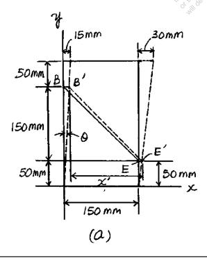
**Ans:**  $(\epsilon_x)_A = 0$   $(\epsilon_y)_A = 1.80(10^{-3}) \text{ mm/mm}$   $(\gamma_{xy})_A = 0.0599 \text{ rad}$   $\epsilon_{BE} = -0.0198 \text{ mm/mm}$
