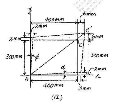
**Ans:**  $(\epsilon_{\text{avg}})_{AC} = 0.0168 \text{ mm/mm}, (\gamma_A)_{xy} = 0.0116 \text{ rad}$
