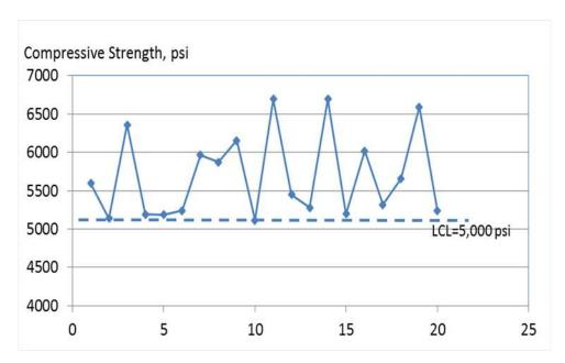
The target value is any value above the specification limit of 5,000 psi. The plant production is meeting the specification requirement.
