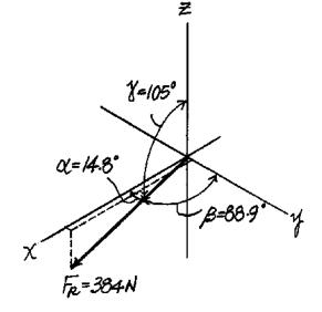
**Ans:**   $F_R = 384 \text{ N}$   $\alpha = 14.8^{\circ}$   $\beta = 88.9^{\circ}$  $\gamma = 105^{\circ}$
