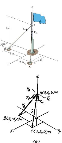
Ans:  $F_R = 1.17 \text{ kN}$   $\alpha = 68.0^{\circ}$   $\beta = 96.8^{\circ}$  $\gamma = 157^{\circ}$
