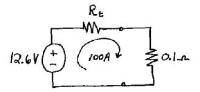
We have  $12.6/(R_f + 0.1) = 100$  from which we find  $R_f = 0.026 \Omega$ . The Thévenin and Norton equivalent circuits are:
