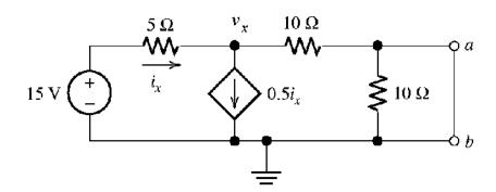
$i_x=\frac{15-v_x}{5}$   $\frac{v_x}{10}-i_x+0.5i_x=0$  Solving, we find  $v_x=7.5\,\mathrm{V}$  and then we have  $i_{sc}=\frac{v_x}{10}=0.75\,\mathrm{A}$ . Then, we have  $R_r=v_{oc}/i_{sc}=6.67\,\Omega$ . Thus the equivalents are:
