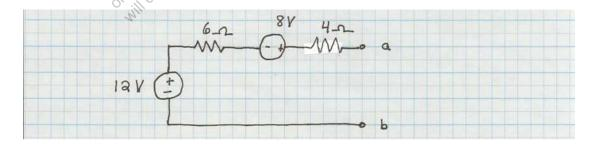
The voltage sources are in series and their voltages can be added. Similarly, the resistances are in series, so we have:
