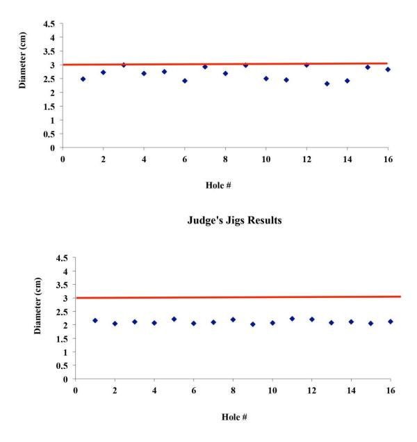
A scatter diagram of the results for Judge's Jigs in the order the holes were drilled shows that on average this machine this machine consistently underdrills and is extremely consistent.
