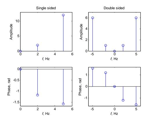
By noting the amplitudes and phases of the various frequency components from the plots, the result is
