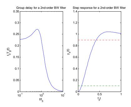
Using the s-shift theorem of Laplace transforms, this inverse transforms to the given expression for the step response (with  $\omega_3 = 2\pi f_3$ ). Plot it and estimate the 10% and 90% times from the plot. From the MATLAB plot of Fig. 2.10,  $f_3 t_{10\%} \approx 0.08$  and  $f_3 t_{90\%} \approx 0.42$  so that the 10-90 % rise time is about  $0.34/f_3$  seconds.
