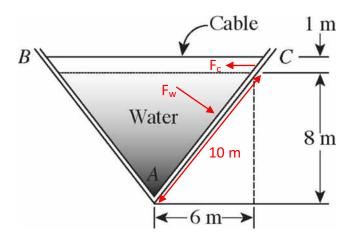
$F_w = \rho_g g \overline{\bar{y}} A = (1000)(9.81)(4)(10)(1) = 392 \text{ kN}$
