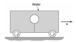
Pressure Gradient is in direction of  $\vec{g}$ - $\vec{a}$  & isobars are perpendicular to  $(\vec{g}$ - $\vec{a})$
