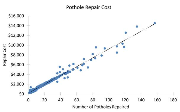
The dotted line is the linear estimation for pothole repair cost. It appears that as the number of potholes in a work order increases, there is more variability in the total cost to repair those potholes. This variability appears to occur around a volume of 40 potholes.
