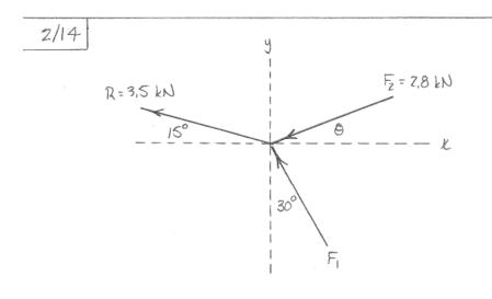
$$\begin{cases} R_{x} = 2F_{x}: -3.5\cos 15^{\circ} = -F, \sin 30^{\circ} - 2.8\cos 0 & 0 \\ R_{y} = 2F_{y}: 3.5\sin 15^{\circ} = F, \cos 30^{\circ} - 2.8\sin 0 & 0 \end{cases}$$
