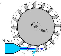
**Discussion** An actual hydroelectric turbine (such as the Pelton wheel) can convert over 90% of this potential to actual electric power.
