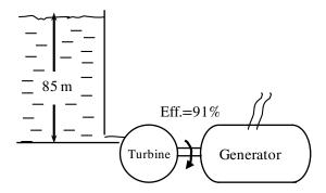
Analysis The total mechanical energy the water in a reservoir possesses is equivalent to the potential energy of water at the free surface, and it can be converted to work entirely. Therefore, the power potential of water is its potential energy, which is gz per unit mass, and  $\dot{m}gz$  for a given mass flow rate. Therefore, the actual power produced by the turbine can be expressed as
