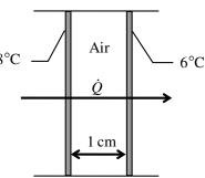
**Properties** The thermal conductivity of air at room temperature is  $k = 0.026 \text{ W/m} \cdot ^{\circ}\text{C}$  (Table 2-3).
