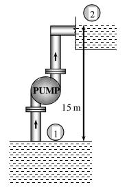
**2-64** Geothermal water is raised from a given depth by a pump at a specified rate. For a given pump efficiency, the required power input to the pump is to be determined.
