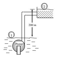
$$\Delta \dot{E}_{\text{mech}} = \dot{m} \Delta e_{\text{mech}} = \dot{m} \Delta p e = \dot{m} g \Delta z = \rho \dot{V} g \Delta z$$
