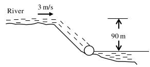
$$e_{\text{mech}} = pe + ke = gh + \frac{V^2}{2} = \left[ (9.81 \text{ m/s}^2)(90 \text{ m}) + \frac{(3 \text{ m/s})^2}{2} \right] \left( \frac{1 \text{ kJ/kg}}{1000 \text{ m}^2/\text{s}^2} \right) = \mathbf{0.887 \text{ kJ / kg}}$$
