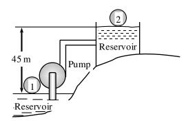
$$\Delta \dot{E}_{\text{mech}} = \dot{m} \Delta e_{\text{mech}} = \dot{m} \Delta p e = \dot{m} g \Delta z = \rho \dot{V} g \Delta z$$
