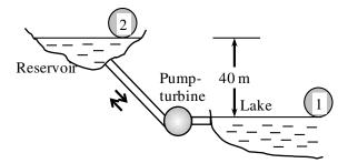
Analysis The total mechanical energy of water in an upper reservoir relative to water in a lower reservoir is equivalent to the potential energy of water at the free surface of this reservoir relative to free surface of the lower reservoir. Therefore, the power potential of water is its potential energy, which is gz per unit mass, and  $\dot{m}gz$  for a given mass flow rate. This also represents the minimum power required to pump water from the lower reservoir to the higher reservoir.
