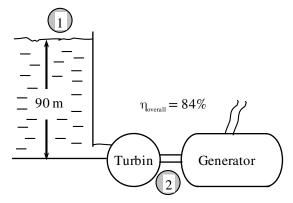
Analysis The total mechanical energy the water in a dam possesses is equivalent to the potential energy of water at the free surface of the dam (relative to free surface of discharge water), and it can be converted to work entirely. Therefore, the power potential of water is its potential energy, which is gz per unit mass, and  $\dot{m}gz$  for a given mass flow rate.
