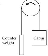
$$\dot{W} = \frac{mgz}{\Delta t} = mgV = (250 \text{ kg})(9.81 \text{ m/s}^2)(1.2 \text{ m/s}) \left(\frac{1 \text{ N}}{1 \text{ kg} \cdot \text{m/s}^2}\right) \left(\frac{1 \text{ kW}}{1000 \text{ N} \cdot \text{m/s}}\right) = 2.94 \text{ kW}$$
