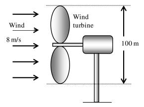
Analysis Kinetic energy is the only form of mechanical energy the wind possesses, and it can be converted to work entirely. Therefore, the power potential of the wind is its kinetic energy, which is  $V^2/2$  per unit mass, and  $\dot{m}V^2/2$  for a given mass flow rate:
