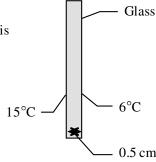
2-93 Prob. 2-92 is reconsidered. Using appropriate software, the effect of glass thickness on heat loss for the specified glass surface temperatures is to be investigated.
