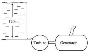
Analysis The total mechanical energy water in a reservoir possesses is equivalent to the potential energy of water at the free surface, and it can be converted to work entirely. Therefore, the power potential of water is its potential energy, which is gz per unit mass, and  $\dot{m}gz$  for a given mass flow rate.
