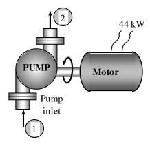
Analysis Then the total mechanical energy of a fluid is the sum of the potential, flow, and kinetic energies, and is expressed per unit mass as  $e_{\text{mech}} = gh + Pv + V^2/2$ . To determine the mechanical efficiency of the pump, we need to know the increase in the mechanical energy of the fluid as it flows through the pump, which is
