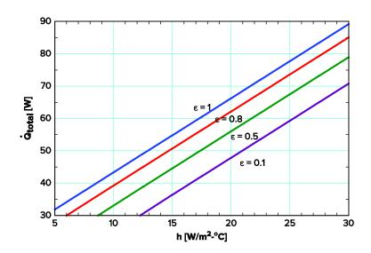
**2-101** A 1000-W iron is left on the iron board with its base exposed to the air at 23°C. The temperature of the base of the iron is to be determined in steady operation.
