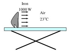
*Analysis* At steady conditions, the 1000 W of energy supplied to the iron will be dissipated to the surroundings by convection and radiation heat transfer. Therefore,
