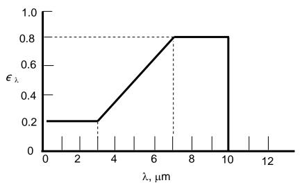
SOLUTION: Numerical or graphical integration is necessary, as no analytical integration appears possible even for this simple variation in spectral emissivity. From Equation 2,10 with  $E_{\lambda b} = \pi I_{\lambda b}$
