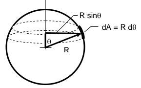
For the sphere, the intercepted energy by a ring element is
