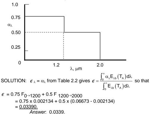
2.7 (a) Obtain the total absorptivity of a diffuse surface with properties given in the figure for incident radiation from a blackbody with a temperature of 6200 K.(b) What is the total emissivity of the diffuse surface with properties given in the figure if the surface temperature is 500 K?
