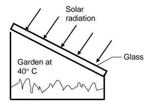
SOLUTION: Part 1;  $\lambda_1 T = 0.38 \ \mu m \ x \ 5780 \ K = 2196.4 \ \mu m \ K$ ;  $\lambda_2 T = 2.7 \ \mu m \ x \ 5780 \ K = 15606 \ \mu m \ K$ . Using Equation 1.37,  $\Delta F = F_{0 \rightarrow \lambda 2T} - F_{0 \rightarrow \lambda 1T} = 0.96951 - 0.10022 = 0.86929$ . The percent transmitted is then 0.86929 x 0.85 x 100 = <u>73.9 %</u>.
