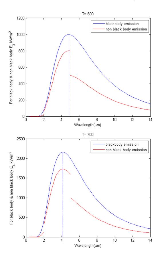
$E_{\lambda}$  is maximum at 2897.8/600=4.83  $\mu m$  which overlaps with the plot.
