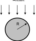
SOLUTION:  $\alpha(\theta) = \epsilon(\theta) = 0.788 \cos \theta$ .  $\rho(\theta) = 1 - \alpha(\theta) = 1 - 0.788 \cos \theta$ . For the cylinder, the intercepted energy on dA per unit length of cylinder is q dA cos  $\theta$  = q (Rd $\theta$ ) cos  $\theta$ , and the reflected energy per unit length is q (Rd $\theta$ ) cos  $\theta$  (1 - 0.788 cos  $\theta$ ). The ratio is
