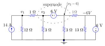
The KCL equation at node  $v_1$ can be written as:
