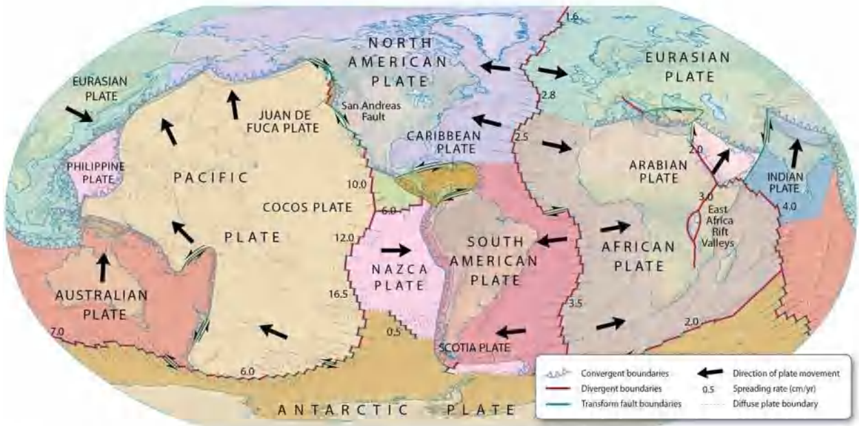
(b) Plate boundaries define the major tectonic plates (shaded), with arrows indicating the direction of motion and numbers representing the rate of motion in centimeters per year.
