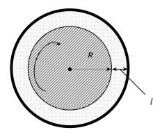
*Analysis* (a) The radius of the shaft is R = 0.05 m, and thickness of the oil layer is  $\ell = (10.3 - 10)/2 = 0.15$  cm. The power-torque relationship is
