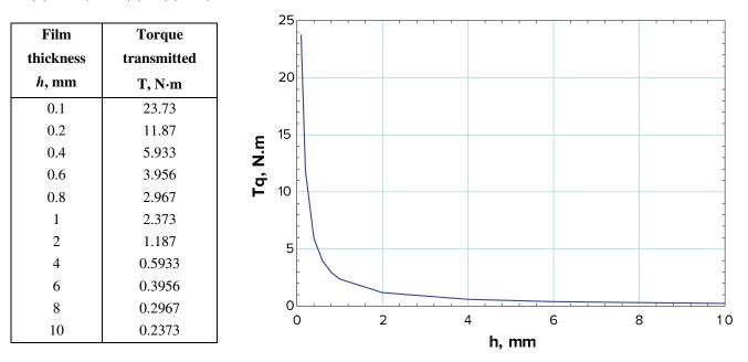
*Conclusion* Torque transmitted is inversely proportional to oil film thickness, and the film thickness should be as small as possible to maximize the transmitted torque.
