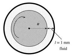
*Assumptions* 1 The inner cylinder is completely submerged in oil. 2 The viscous effects on the two ends of the inner cylinder are negligible. 3 The fluid is Newtonian.
