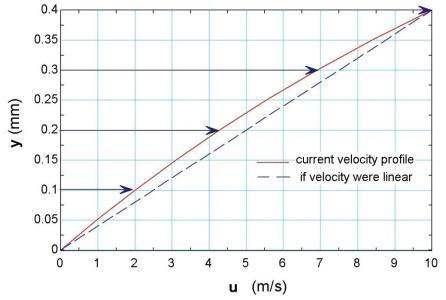
(b) Using Newton's law of viscosity
