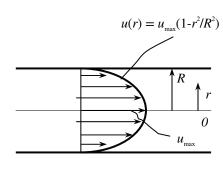
**Solution** The velocity profile for laminar one-dimensional flow through a circular pipe is given. A relation for friction drag force exerted on the pipe and its numerical value for water are to be determined.
