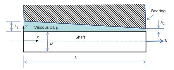
The varying clearance h can be expressed as a function of axial coordinate x (see figure). According to this sketch we obtain
