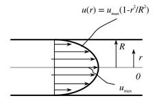
Note that the quantity du/dr is negative in pipe flow, and the negative sign is added to the  $\tau_w$  relation for pipes to make shear stress in the positive (flow) direction a positive quantity. (Or, du/dr = -du/dy since y = R - r). Then the friction drag force exerted by the fluid on the inner surface of the pipe becomes
