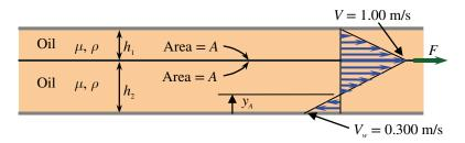
Equating triangles, we know that u = 0 at  $y = y_A$ , where  $y_A / V_w = h_2 / (V_{\text{plate}} + V_w)$  or  $y_A = V_w h_2 / (V_{\text{plate}} + V_w)$ . Plugging in the numerical values, we get  $y_A = (0.300 \text{ m/s})(1.65 \text{ mm})/(1.00 + 0.300) \text{ m/s} = 0.381 \text{ mm}$ .
