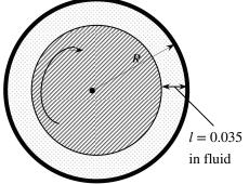
*Assumptions* 1 The inner cylinder is completely submerged in the fluid. 2 The viscous effects on the two ends of the inner cylinder are negligible. 3 The fluid is Newtonian.
