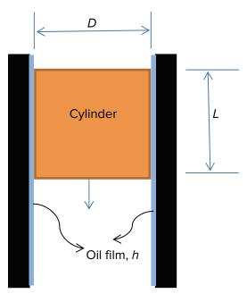
Analysis Assuming a linear velocity profile in the oil film the drag force due to wall shear stress can be expressed as
