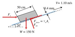
**Solution** For flow over a plate, the variation of velocity with distance is given. A relation for the wall shear stress is to be obtained.
