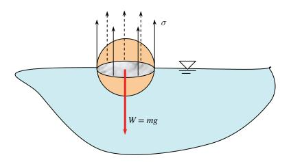
Analysis The surface tension force and the weight of the ball can be expressed as
